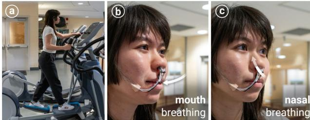
**Figure 13:** (a) A user does cardio while wearing our device. (b) Normally, they inconsistently breathe through the nose and, instead, breathe through the mouth, but (c) at times, our device encourages nasal breathing by increasing the perceived airflow when they inhale nasally.
